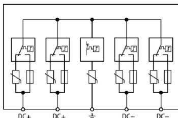
Basic circuit diagram DCU YPV SCI 1000 2M
