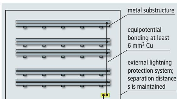
Figure 1 Functional earthing of the mounting systems if no external lightning protection system is installed or the separation distance is maintained (IEC TR 63227)
