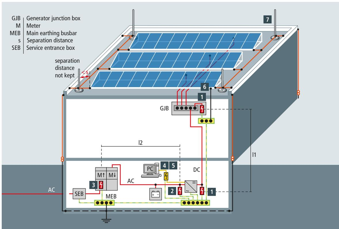
Figure 15 PV system installed on a building with external LPS and insufficient separation distance
