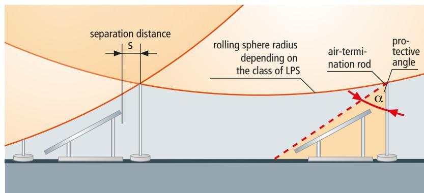
Figure 13 Rolling sphere method versus protective angle method for determining the protected volume
