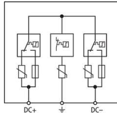
Basic circuit diagram DCU YPV SCI 1000 1M
