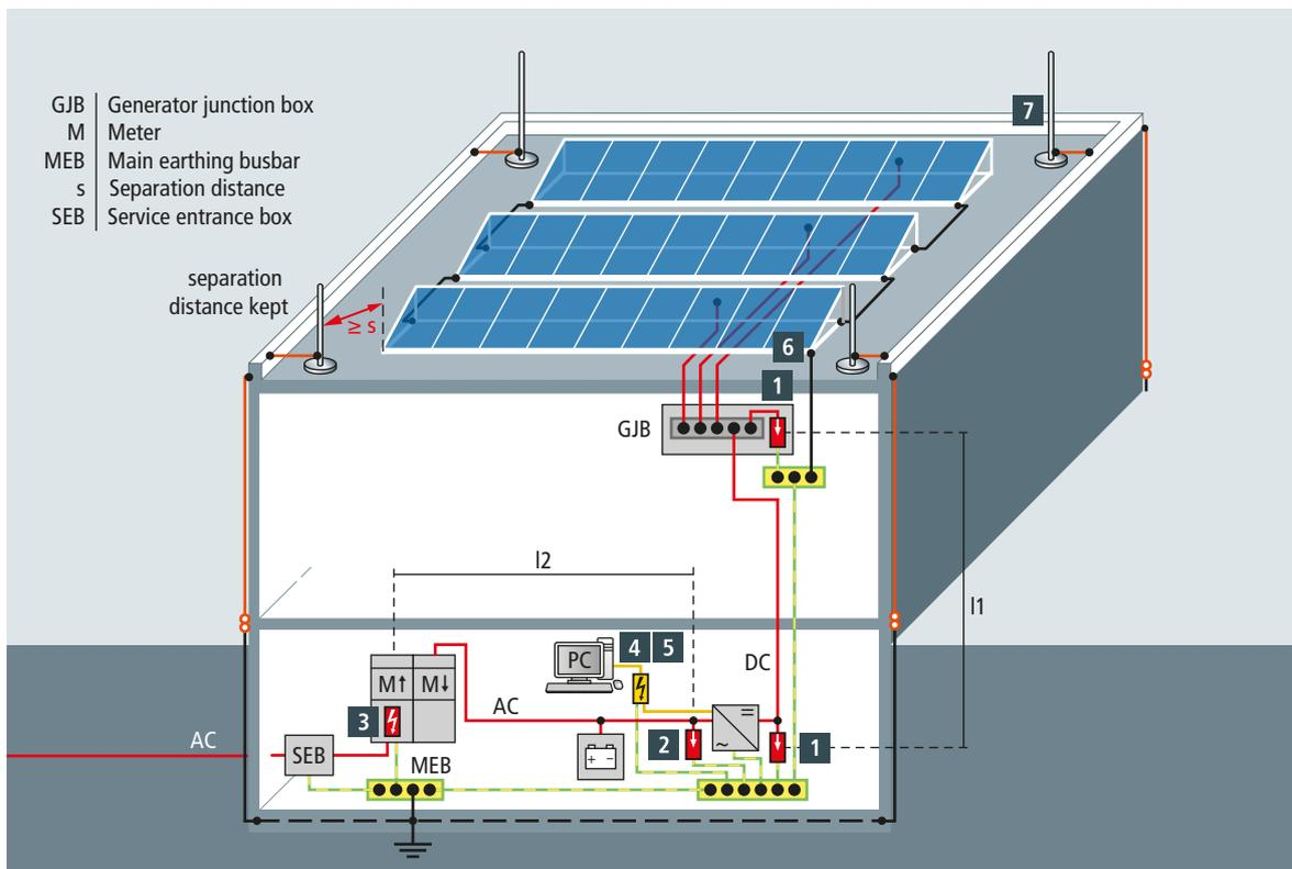
Figure 11 PV system installed on a building with external LPS and sufficient separation distance Table 5 of IEC 62305-1 (EN 62305-1)
