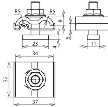
Earthing clamps for integrating mounting systems, e.g. of PV installations in the functional equipotential bonding/functional earthing (black conductor possible) and lightning equipotential bonding according to IEC/EN 62305-3.
