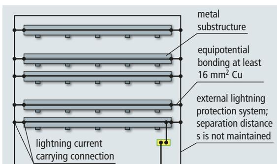
Figure 2 Lightning equipotential bonding for the mounting systems if the separation distance is not maintained
